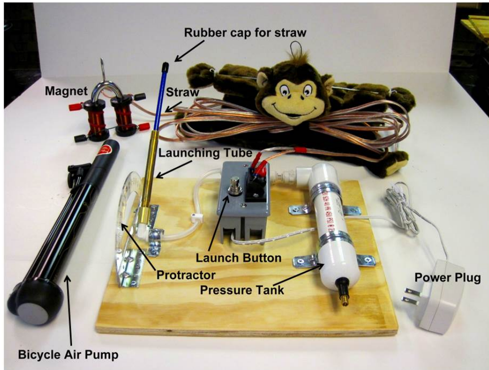
Figure 6. The straw rocket launcher included in this unit (tank safety valve not shown).
