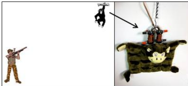
Figure 8. Monkey and zookeeper scenario and setup: electromagnet hanger-metal rod on monkey, hanging on wall.
