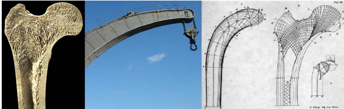
Figure 5. Left: cross section of human femur, showing trabeculae; Center: Fairbairn crane; Right: Cullmann's and von Meyer's drawings of stress patterns in a Fairbairn crane and trabecular alignment in the femur.
