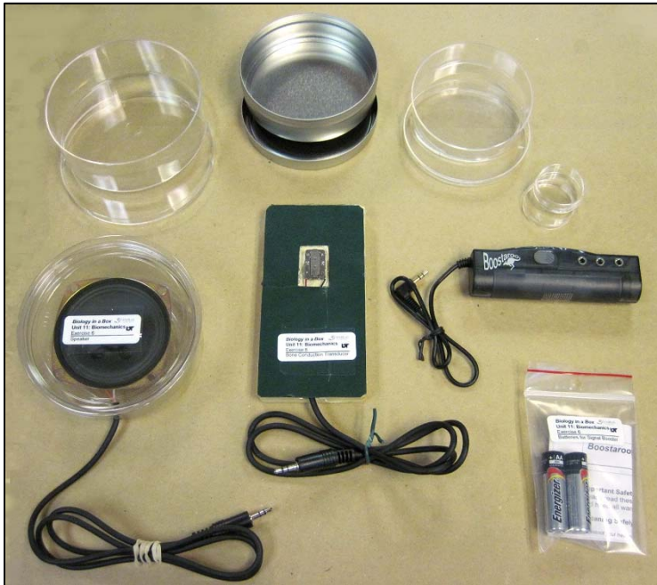
Figure 2. Items required for use in Exercise 6e Crank it up! Top row offers a variety of diaphragms. Bottom row from left to right: Speaker (protected in clear 8oz deli cup with audio cable soldered on), Bone Conduction Transducer (embedded in wood block with audio cable soldered on), and Mini Signal Amplifier (Boostaroo) with batteries.
