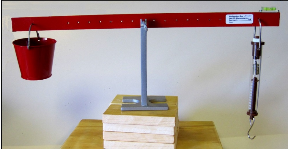
Figure 4. Apparatus for testing the mechanical advantage of a Class 1 lever.
